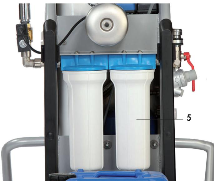
Unscrew the filter container of the 5µm filter (5).
